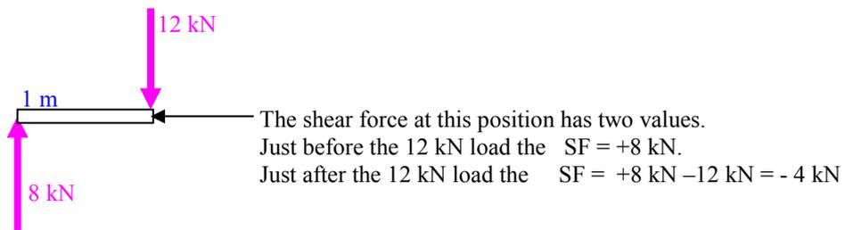
Continuing to the end of the beam at the RHS, the SF will remain constant at -4 kN.
