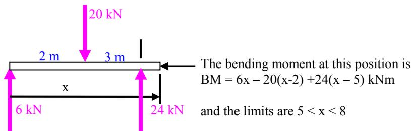
Substituting values for  $x$  and plotting the complete diagram gives:
