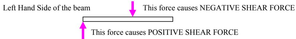
Values of SF can be found at different distances along the length of the beam and if necessary used to plot a graph.
