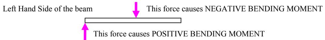
If a **POSITIVE BENDING MOMENT** is acting on the beam it causes **SAGGING**.
