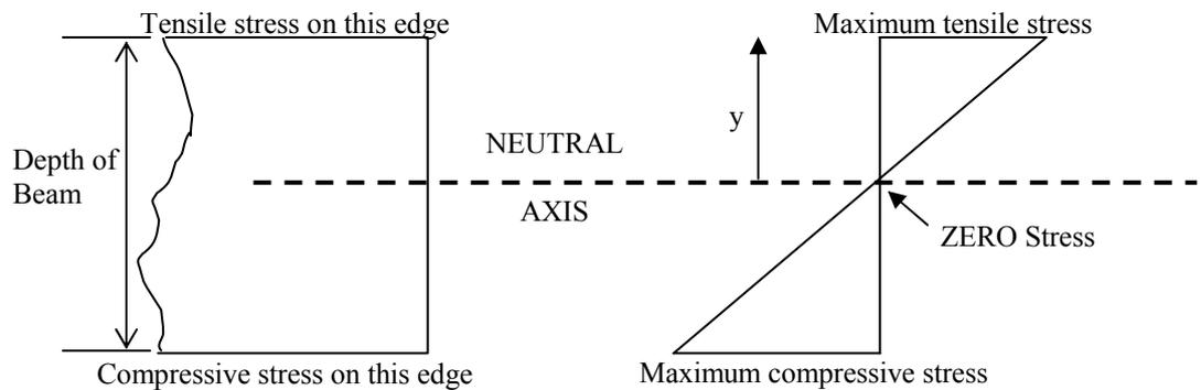
For symmetrical or simple shapes, the position of the Neutral Axis is easy to find since it passes through the CENTROID of the shape.
