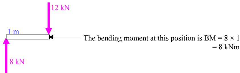
Very often an equation is needed to find the BM at any value of  $x$  (distance along the beam). Once the equation has been established, any value of  $x$  can be substituted and the BM found. The difficulty is that a new equation is needed every time there is a load change.
