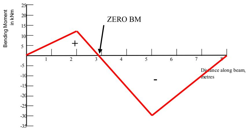
Again, the maximum positive BM of +12 kNm and the maximum negative BM of -30 kNm occur where the SF is zero.
