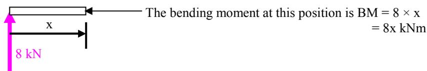
Now any value of  $x$  between 0 and 1 m can be substituted into  $8x$  to give the bending moment at that position.
