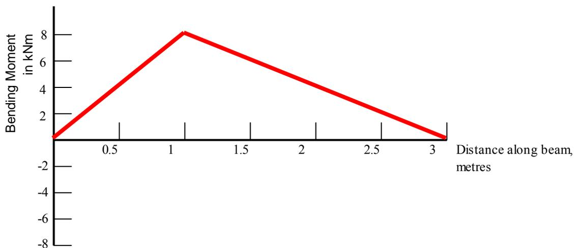
In this example all the bending moment diagram is positive, which means the beam will be sagging.
