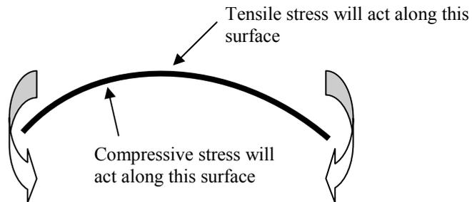
It can be shown that an equation relating Bending Moment  $M$  to Bending Stress  $\sigma$  is given by:
