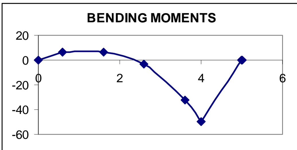
The final part of the question asks for the point of contraflexure. i.e. where the Bending Moment is zero. From a rough sketch of the BM diagram, this will occur within the UDL part of the beam.
