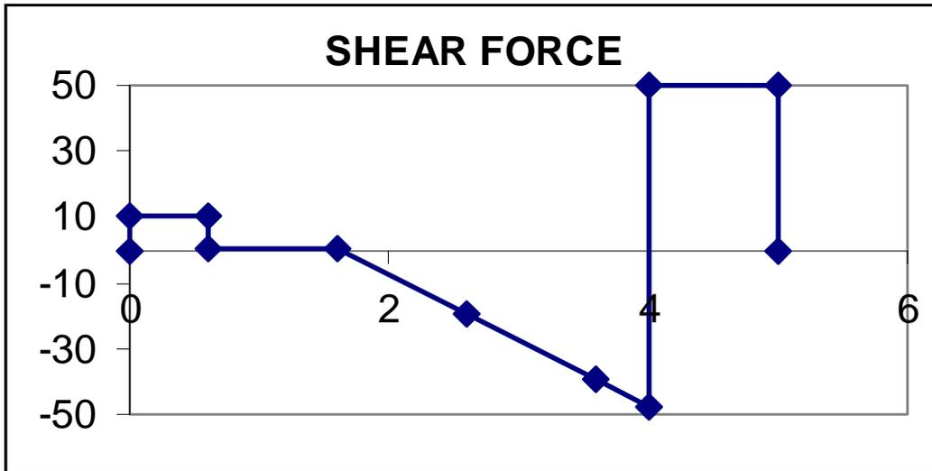
The maximum bending moment can also be found. The maximum bending moment will ALWAYS be at the point where the shear force is zero, so we only need to find the bending moment at two points.
