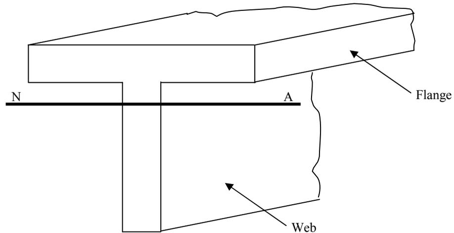
A datum line is needed about which to take moments. This is usually the base line of the cross section. The cross section is then subdivided into simple shapes whose area and own neutral axis can be found. In this example, the cross section is subdivided into two rectangles.
