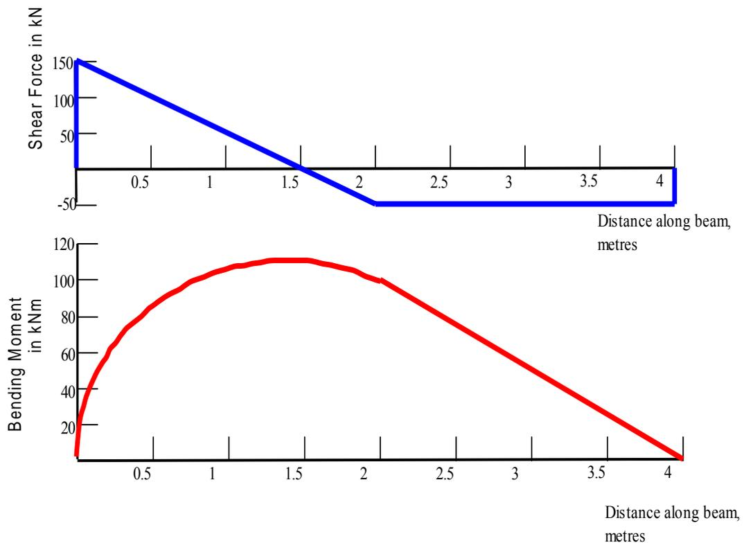
The maximum bending moment again occurs where the shear force is zero. The diagram shows that the shear force is zero between 0 and 2 m. Therefore, using the correct equation for shear force the exact position of maximum bending moment can be calculated.
