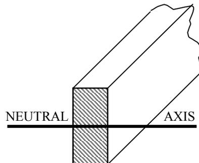
For more complicated shapes the position needs to be found using **FIRST MOMENTS OF AREA**. An example could be a beam which has a T for the cross sectional shape.
