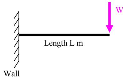
At the wall, there must be a vertical reaction force to support the load  $W$ . In addition there is a **FIXING MOMENT** which prevents rotation of the beam caused by the moment  $WL$ .
