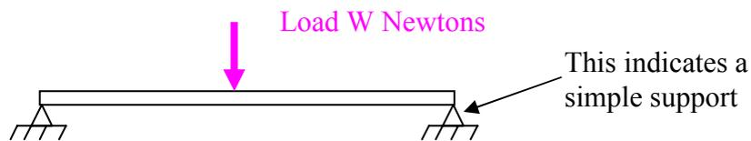
The load and reaction forces at the supports cause shear forces in the beam.
