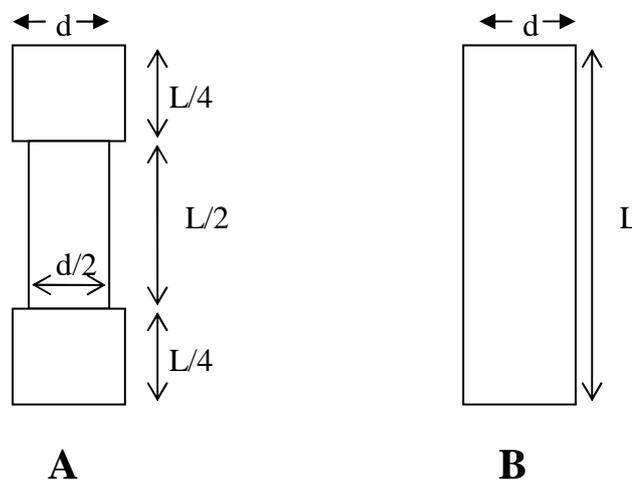
$$\text{Resilience} = \text{Strain Energy Stored} = \frac{\sigma^2 \times \text{volume}}{2E}$$
