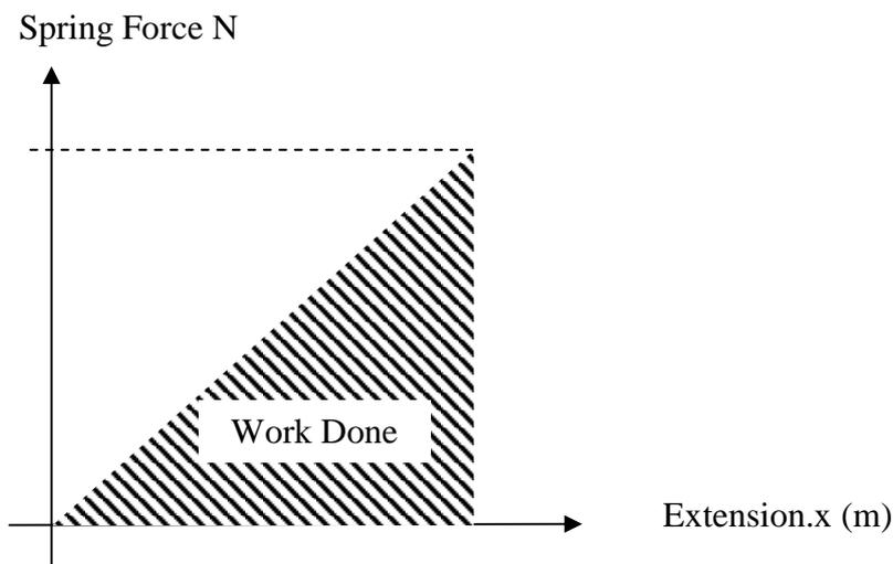
This shows that the work done =  $\frac{1}{2} Px$  (or  $\frac{1}{2} kx^2$ ), based on the fact that the average load on the spring is
