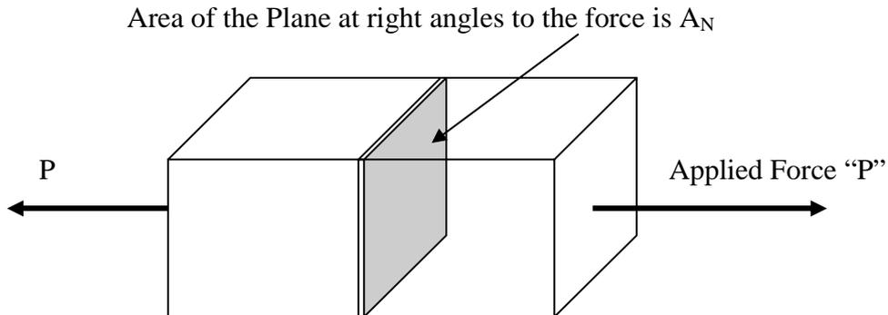
If we now consider a plane at some other angle  $\theta$  to the normal, then the load can be resolved into two mutually perpendicular directions, parallel and normal to the plane. The component normal to the oblique plane will cause a direct stress  $\sigma_0$ , whilst that parallel to the plane will cause a shear stress  $\tau$ .
