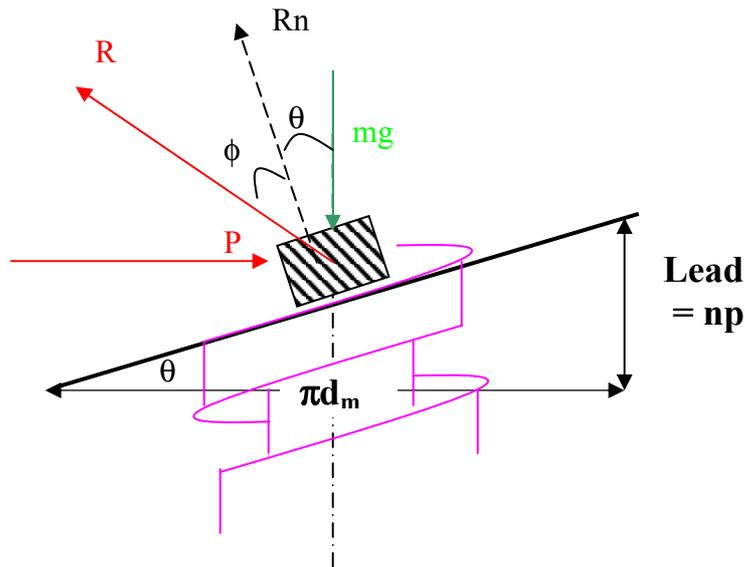
The small shaded block represents a portion of the nut on the sliding thread.
