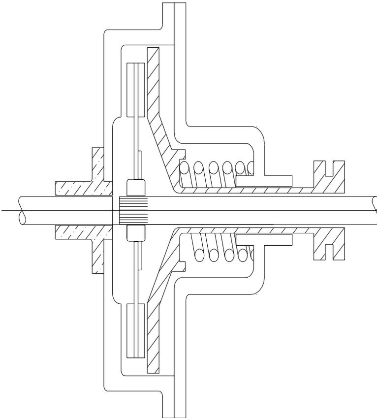
Use is made of expendable friction material (Compound Asbestos Fibre being common). The force holding the plates together enables a friction torque to be transmitted from one shaft section to the other. Use of such a clutch gives a smooth take up of power and sudden torque surges are eliminated. Additionally, such a clutch can be used as a torque limiting device.
