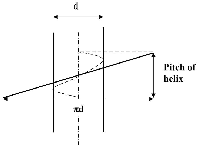
The square screw thread can be regarded as such a helix and can be developed as an inclined plane. The inclined plane formed will have a base of length  $\pi d$  where  $d$  is the mean diameter of the thread. The height of the plane is the lead of the thread, which is the number of starts "n" times the pitch.
