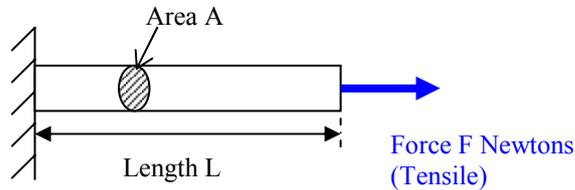
The stress,  $\sigma$ , is given by  $\frac{\text{force}}{\text{area}}$  and the units are  $\text{N/m}^2$ . Therefore  $\sigma = \frac{F}{A}$
