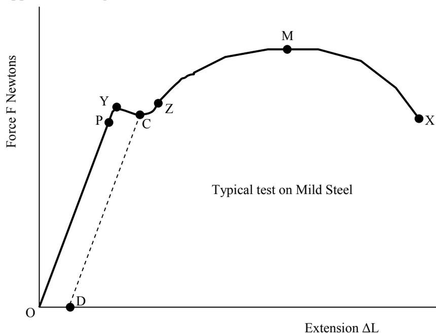
The **Elastic Stage** is when the component is unloaded and it returns to its original unstretched length. This is represented by the line OP, and the material is said to obey Hooke's Law.
