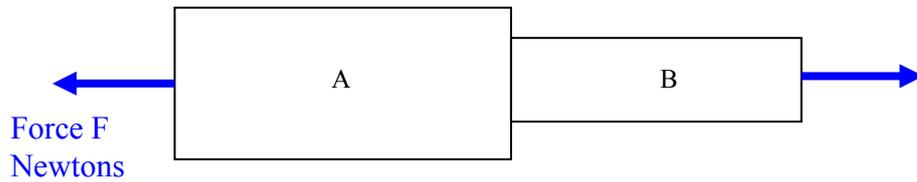
The two components A and B may be different materials (e.g. one steel and one copper), they may be different lengths, they may be different cross sectional areas.
