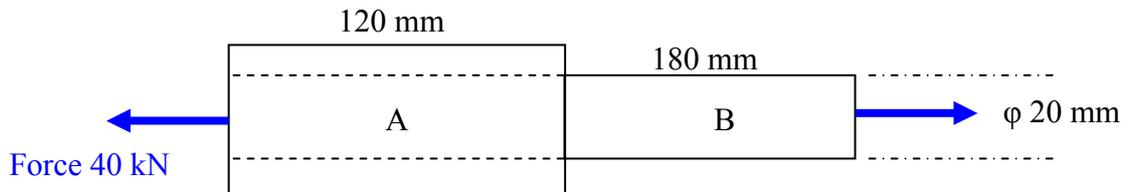
The question says that  $\sigma_A = \sigma_B$ . Therefore  $\frac{F}{A_A} = \frac{F}{A_B}$  and since the force applied to each component is the same then the areas must be equal i.e.  $A_A = A_B$ . If the outside diameter of component A is said to be 'D' then
