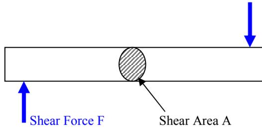
The Shear Stress,  $\tau$ , is given by  $\frac{\text{shear force}}{\text{shear area}}$  and units are  $\text{N/m}^2$ . Therefore  $\tau = \frac{F}{A}$
