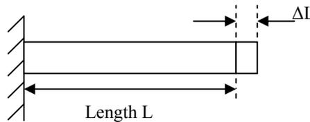
The strain,  $\epsilon$ , is given by  $\frac{\text{change in length}}{\text{original length}}$  and there are no units. Therefore  $\epsilon = \frac{\Delta L}{L}$
