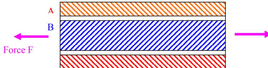
The force  $F$  is now shared between the two components. The problem is how much of the force is taken by component A and how much is taken by component B. Whatever the value, both added together must equal the total force  $F$ .
