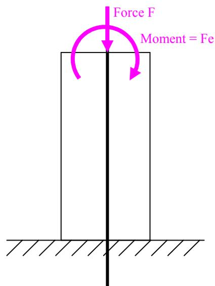
The direct stress will be given by  $\sigma = \frac{F}{A}$  and will be compressive.
