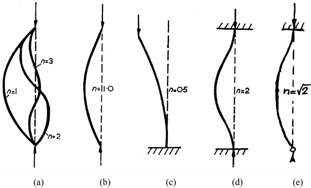
Diagram (a) shows a strut pin jointed at each end. There are several modes of failure as illustrated, but it is the smallest value of load, and therefore  $n$ , which will cause failure. In this case the failure will be when  $n = 1$  as in diagram (b).
