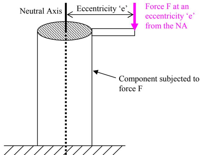
The component has a force F Newtons applied to it, which, in this drawing, is offset from the Neutral Axis by an eccentricity 'e' metres. This force causes both a direct compressive stress in the component and also a bending stress due to the moment 'Fe' Nm.
