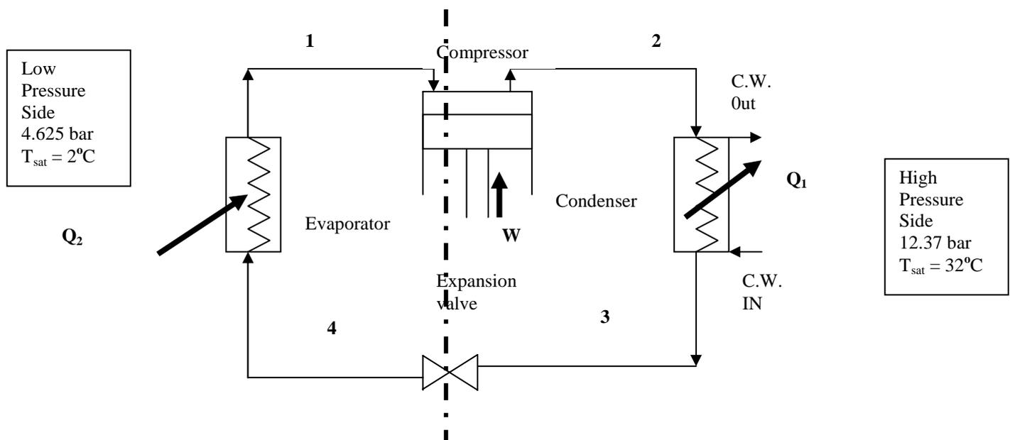
Draw the TS and ph diagrams ensuring the relevant diagram positions for the fluid states. i.e. saturated liquid at exit from the condenser and saturated vapour at exit from the evaporator
