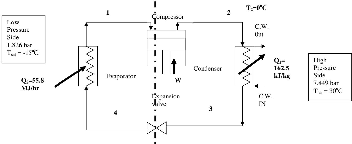
$T_1 = 0^\circ\text{C}$   $\therefore$  refrigerant has  $15^\circ\text{C}$  of superheat
