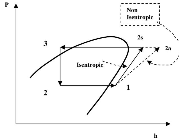
We have previously defined the CARNOT coefficient of performance (C.O.P.) for the refrigeration and heat pump system. With actual cycles it is usually possible to determine the enthalpies at the cardinal points of the cycle and thus determine the actual C.O.P. required. This Actual C.O.P. can be defined in terms of those enthalpies.
