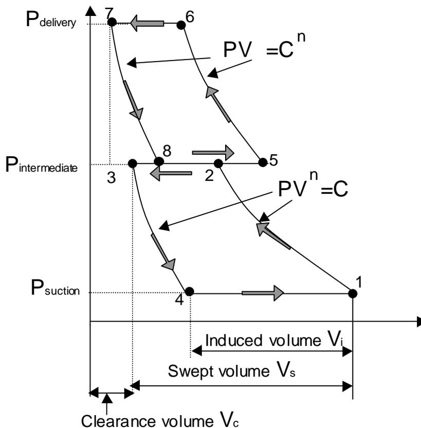
In this diagram it is assumed that the delivery process from the first or LP stage and the induction process of the second or HP stage are at the same pressure.
