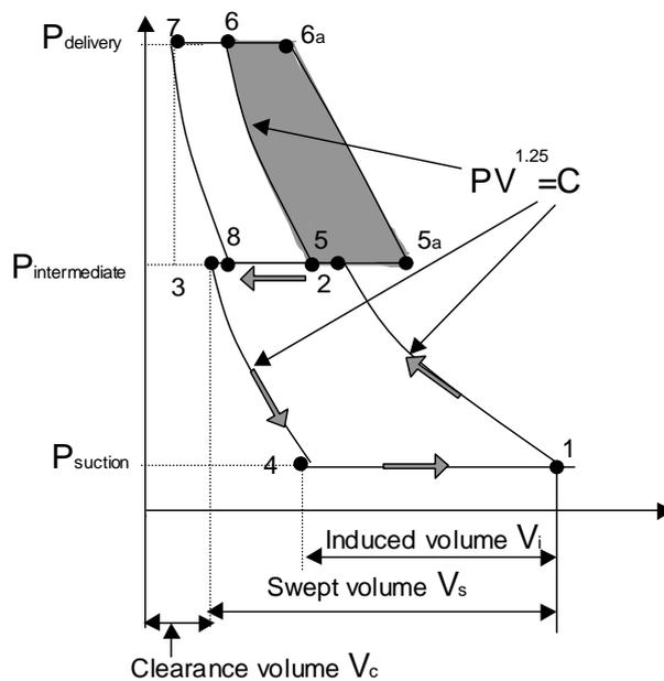
The power saved by inter-cooling is that shown shaded on the second stage portion of the diagram and is the difference between the second stage powers calculated at the different inlet temperatures.
