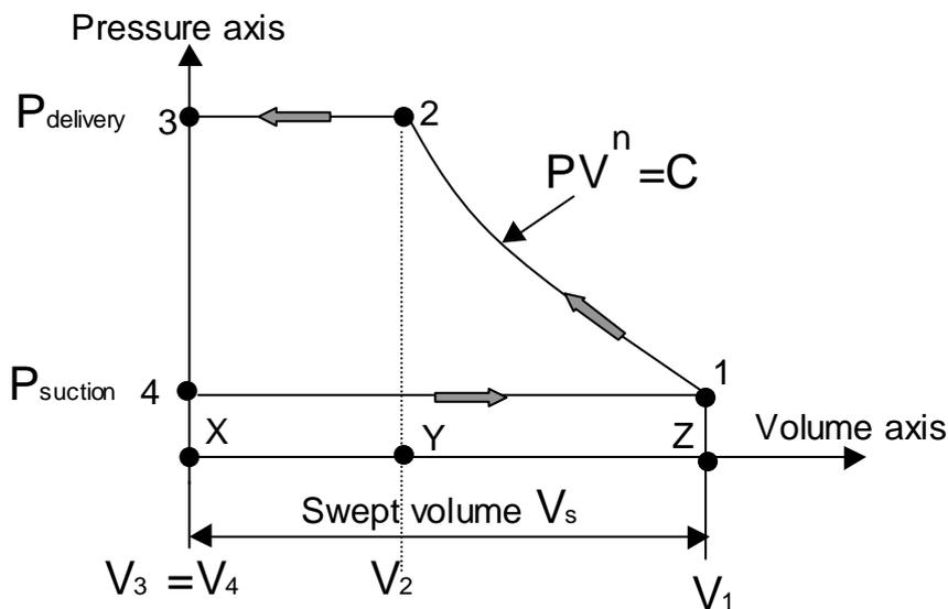
The indicator (PV) diagram shown above represents the ideal case in which the air in the cylinder is considered a perfect gas and all processes are reversible.
