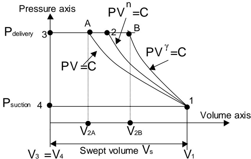
This diagram shows the limits of the possible values of  $n$  which also shows that  $V_2$  can vary from a maximum of  $V_{2B}$  to a minimum of  $V_{2A}$ .
