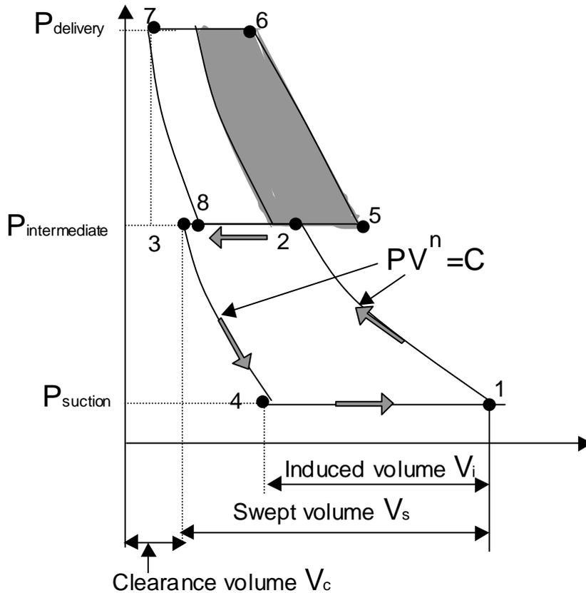
The two indicator diagrams 1234 and 5678 are shown with a common pressure,  $P_{intermediate}$ . This does not occur in a real machine as there is a small pressure drop between the cylinders however this can be ignored in test examples. An after-cooler can also be fitted after the delivery process to cool the gas.
