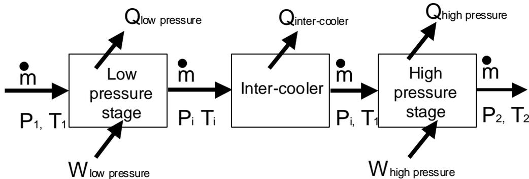
The above diagram shows steady flow through a two stage-reciprocating compressor with inter-cooling.
