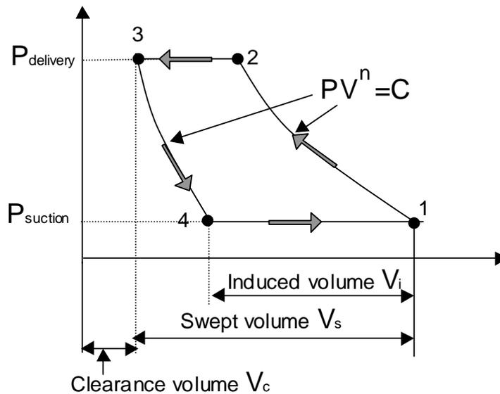
In this case when the piston is at top dead centre the clearance volume  $V_c$  is full of gas at pressure  $P_2$  and temperature  $T_2$ .
