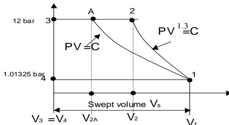
This diagram shows the two conditions, The actual compression 1 to 2 and that for the isothermal compression 1 to A.
