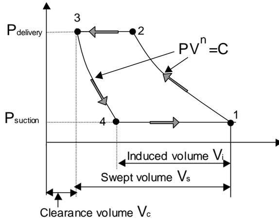
To obtain the compressor speed we need to calculate the amount of air delivered per cycle which is the induced volume  $V_1 - V_4$ .
