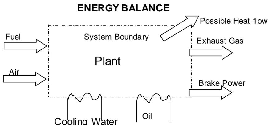
$$\dot{Q} - \dot{W}_{bp} = (\dot{m}_a + \dot{m}_f)c_{p(gas)}(T_2 - T_0) - \dot{m}_a c_{p(air)}(T_1 - T_0) - \dot{m}_f c_{p(fuel)}(T_1 - T_0) - \dot{m}_f CV + \dot{m}_{cw} c_{p(cw)} \Delta T_{cw} + \dot{m}_{oil} c_{p(oil)} \Delta T_{oil}$$
