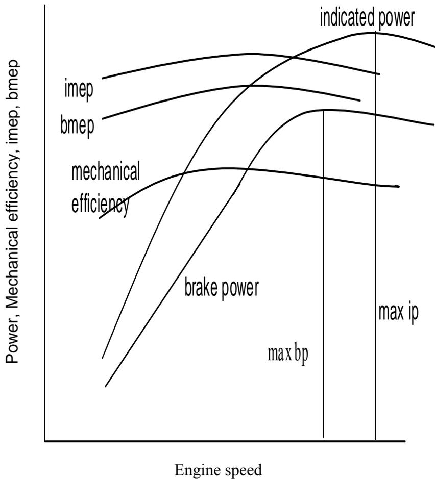
Consider the indicated power and brake power curves, as the speed increases from the lower values the two curves deviate since the friction power increases with speed, both curves show maximum values, but they occur at different speeds.
