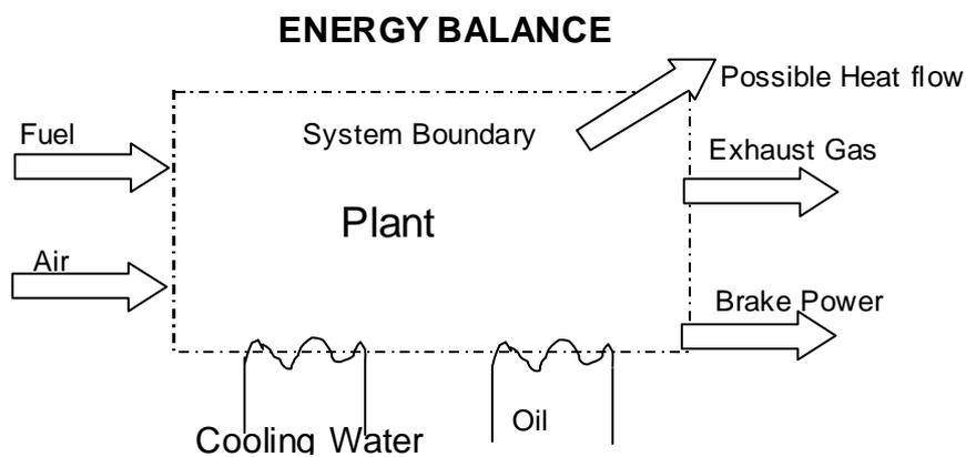
The boundary is drawn around the system to include to the effects considered relevant. The steady flow energy equation is then written for the system.
