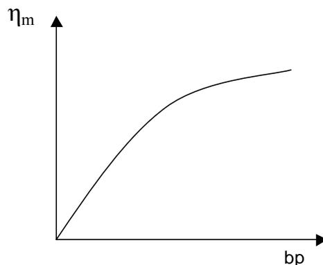
At zero bp at the same speed the engine is developing just sufficient power to overcome the frictional resistance.
