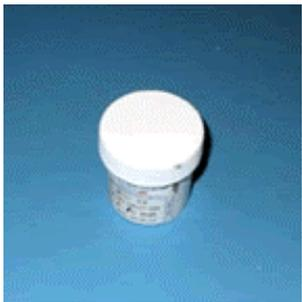
**Solder Paste:** There are lots of solder paste manufacturers. Some don't provide printable paste in containers less than 500 gr. For a small number of PCBs this would be expensive. What you want is standard eutectic tin/lead solder. This is typically available in either small jars or in the syringes that are typically used in rework stations. Most vendors providing home prototype stencils will have small jars of solder
