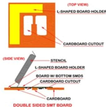
Tape the cardboard "holder" to the work table and do everything on top of the cardboard the same as you did when screening solder paste on the first side. The reflowed components nest safely in the openings in the cardboard. The board rests flat on the cardboard with the surface to be screened is open to the prototype stencil.
