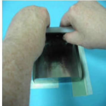
Inspect the solder paste print to ensure all the lands have solder paste on then and the paste is not smeared. If the print is not good, immediately use a spatula to remove the solder paste from the PCB. Clean the paste that remains on the PCB with alcohol and a clean rag. Let the PCB dry and print the solder paste again.
