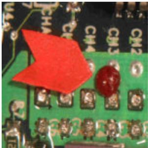
When the temperature indication mark melts, remove the board from the oven. Be careful not to disturb the molten solder joints. Place the board on a surface and let it cool to near room temperature. Inspect the solder joints. Use
