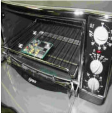
Important: Before reflowing starts, turn the oven on to heat up, a minimum of five minutes. Set the oven to bake and set the temperature to the highest baking temperature setting (450 to 500 degrees F).
