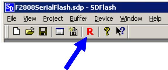
NOTE: The reset button of SDFlash Serial CANNOT reset the DSP target. If the target is in a bad state or not in bootloader mode then user must use a hardware reset to get target back to bootloader mode (per step 12). Once that is done the reset button is used to inform SDFlash that target is in bootloader mode.
